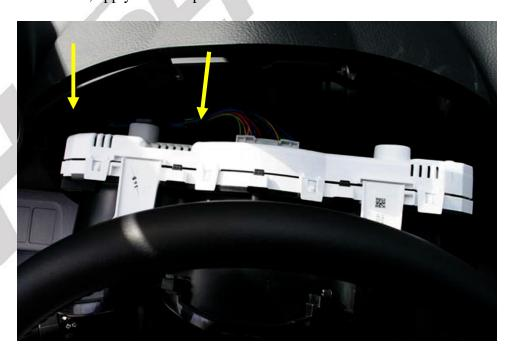
5. Connect the male end of the Speedometer Calibrator Harness to the factory wiring harness.
