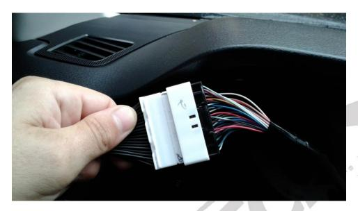
6. Connect the female end of the Speedometer Calibrator Harness into the Instrument Cluster.
